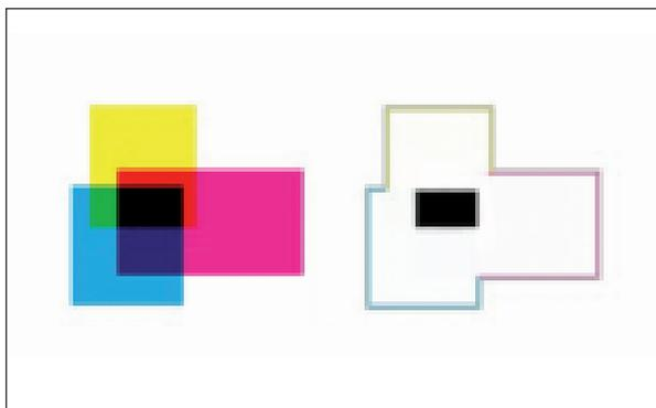
Fig. 2: basic CMY forming visual neutral response, and possible replacing with black domain.
