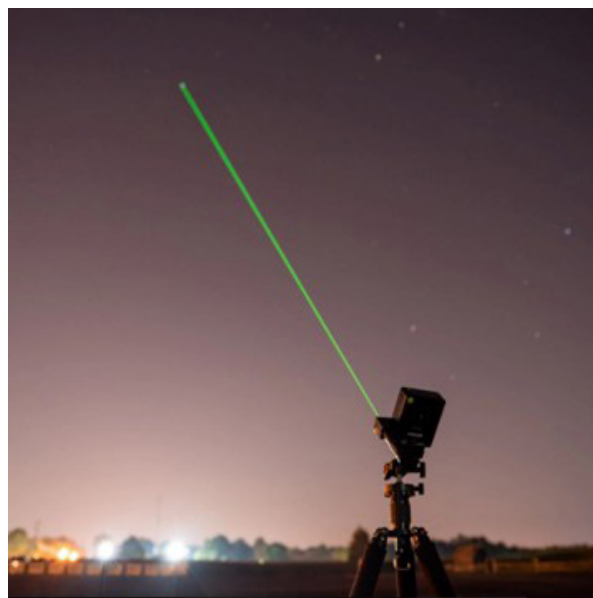
Figure 3 Small portable tracker MoveShootMove that does polar alignment [5]
