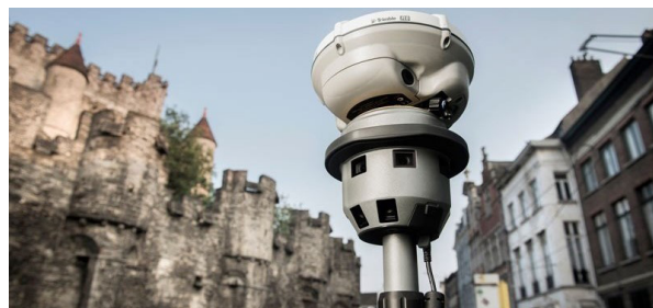
Slika 4 Prikaz terestričke kamere Trimble V10 Imaging Rover Figure 4 Illustration of the Trimble V10 Imaging Rover terrestrial camera (Izvor: https://allterra-hungary.com/termek/v10/ )
