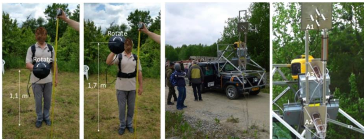
Figure 1: a), b) Manual survey includes search in the vertical and horizontal plane, after signal detection of IED, rotation of antenna matches the polarization, [1], [2]. c) Harmonic radar in development for IED detection from ground vehicles, b) antennas, NATO, [7].
